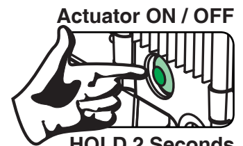
HOLD 2 Seconds Figure 2: Powering ON the actuator
